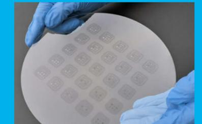
2GL enables the fabrication of master templates for subsequent replication processes, such as nanoimprint lithography (NIL) and micro injection molding ( $\mu\text{IM}$ ). It is also ideal for rapid prototyping of designs that can be directly validated for the requirements of the microoptics industry.
